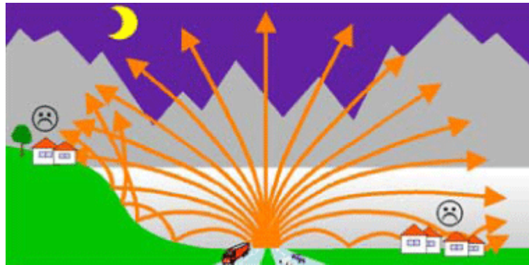
Figure 26: Direction of sound spreading (sound rays) during night
