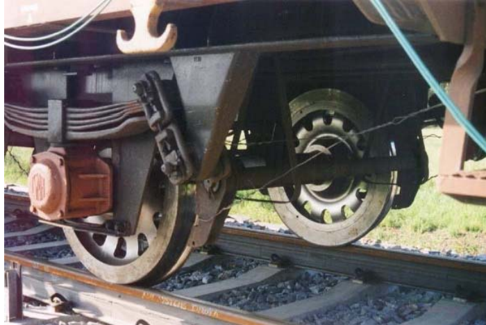
Figure 12: Ring damped and perforated wheel
